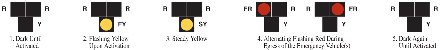
FY -Flashing Yellow • SY -Steady Yellow • FR -Flashing Red OPTION: A "Steady Red" clearance interval may be used after a "Steady Yellow."
