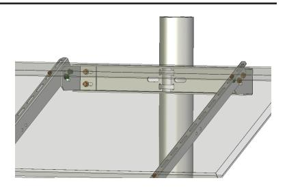
2. Attach the clips to the bucket. In each of the 4 mounting holes, use a bolt and flat washer on one side, and a washer, lock washer and nut on the other.
