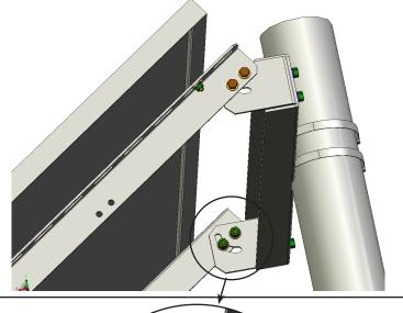
3. If desired, loosen the bolts holding the rails to the clips, and adjust the tilt of the panel as required
