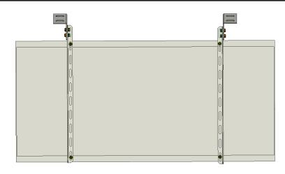
If the distance between the PV module mounting holes is 26.9" or more, attach the clips to the rails so the protruding end of the clips are facing the the center of the module.
