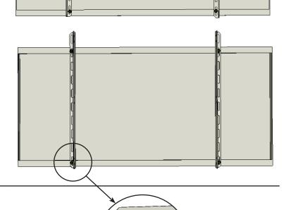
2. Secure the rails with a bolt, lock washer and hex nut in each of the 4 mounting holes.
