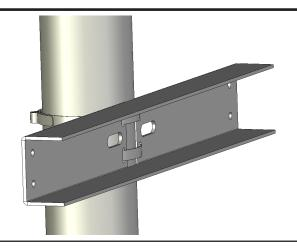
2. Tighten the hose clamp screws to 70 inchlbs.
