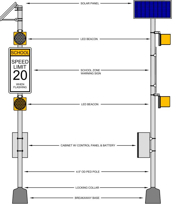
Figure 1 - Typical Traffic Warning Solar System (School Zone)
