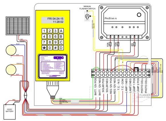
Figure 2 - Standard Control Panel Schematic (School Zone)
