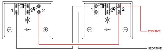
Figure 9 - Two Type 'G' Junction Boxes in Parallel
