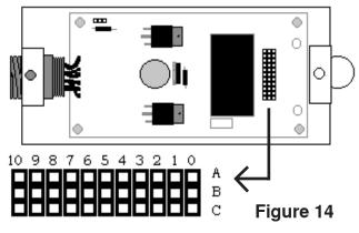
Tables 1 and 2 show the jumper settings for each option. Table 1 contains the general pin settings and Table 2 contains the flash rate pin settings.
