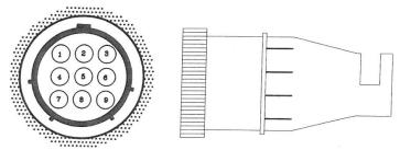
Figure 5 - Female Backbone CPC END (Attached to Solar Panel, Battery, and LED Wires)
