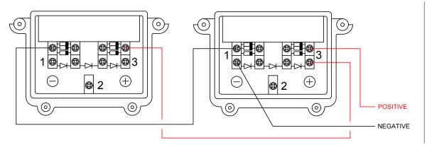
Figure 8 - Two Type 'M' Junction Boxes in Parallel
