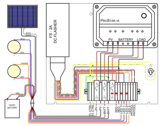
Figure 3 - Standard 24-Hour Control Panel Schematic
